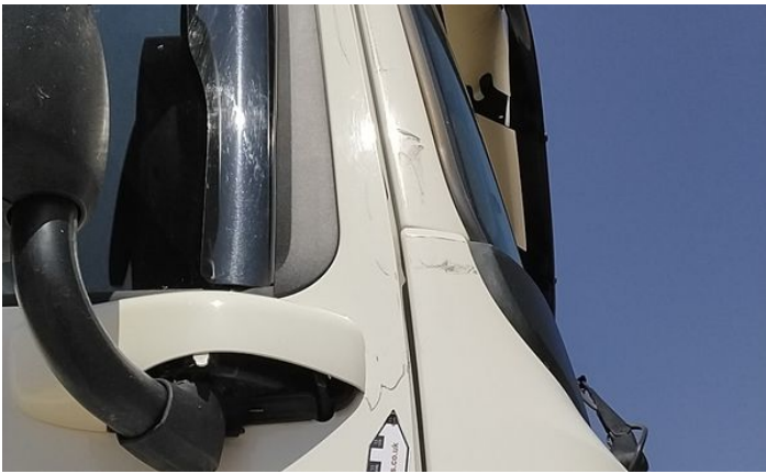
9: Qtr Panel osr Rusted Over 5mm
