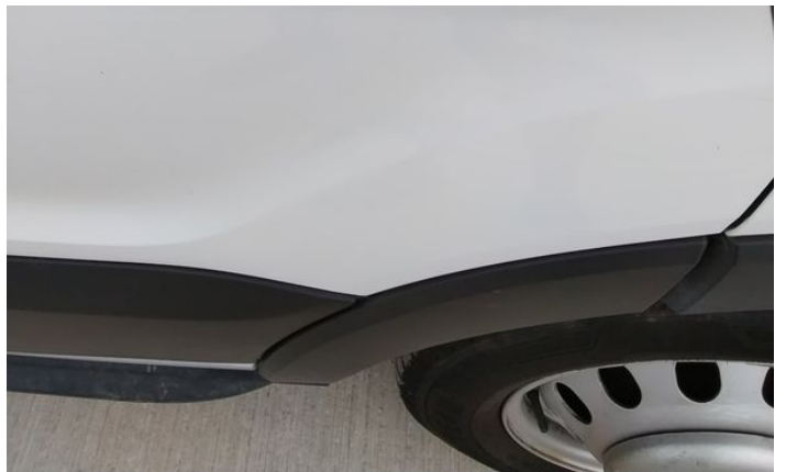
12: Sill Panel Trim os Missing Replace
