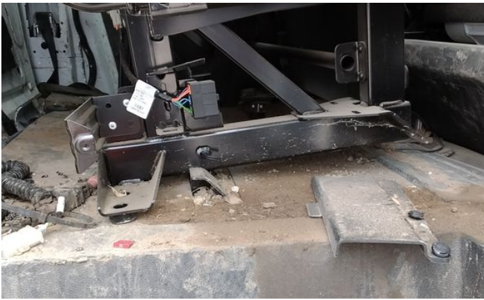
21: Seat Belt nsr Broken Replace
