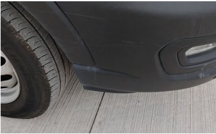
15: Wing osf Scratched Over 25mm Thru Paint
