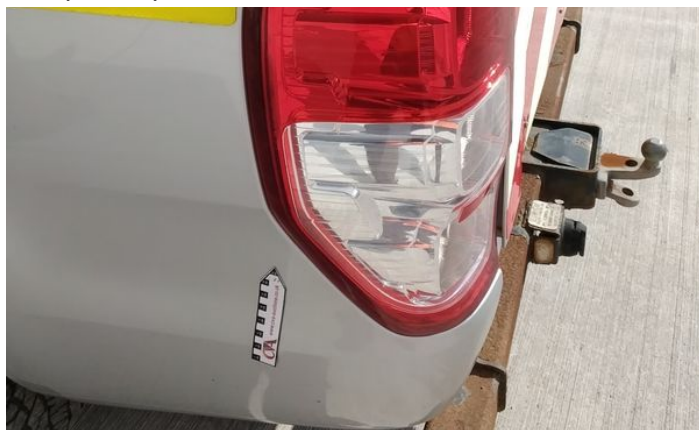
6: Qtr Panel nsr Chipped Multiple Chips
