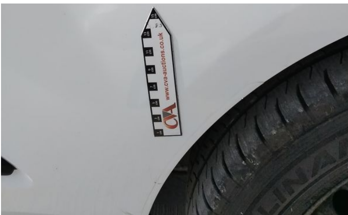
17: Qtr Panel osr Dented Over 30mm
