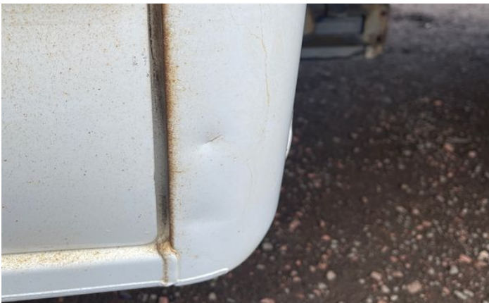
11: Qtr Panel nsr Dented With Paint Damage
