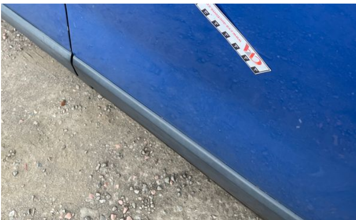
5: Sill os Poor Previous Repair Paint Flake
