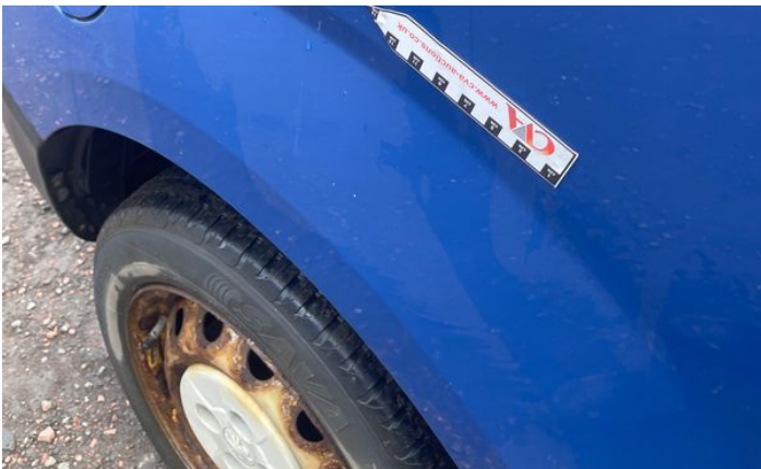
5: Wing osf Rusted Over 5mm
