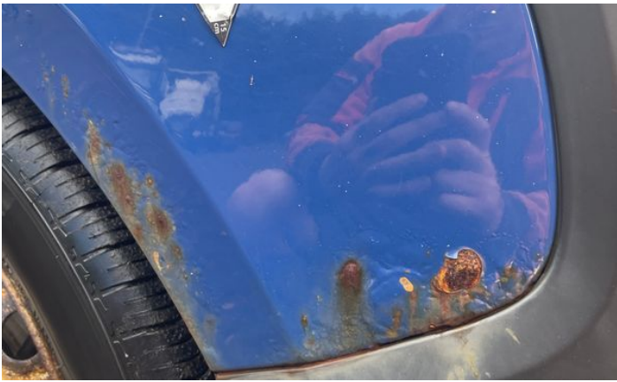
3: Sill os Rusted Over 5mm
