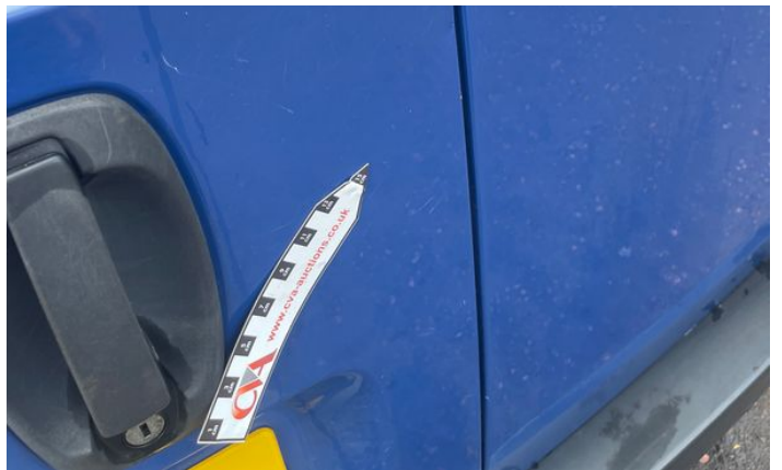
6: Door osf Dented Over 30mm
