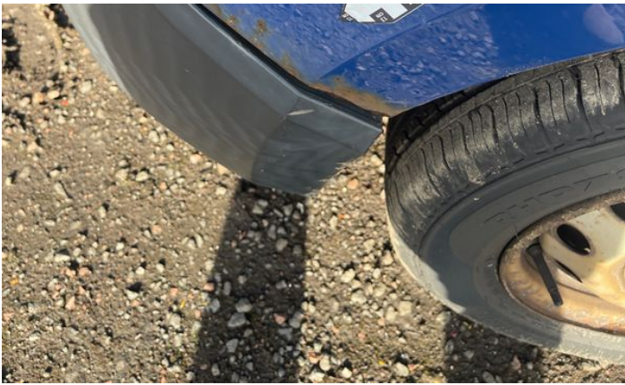
9: Sill ns Dented With Paint Damage
