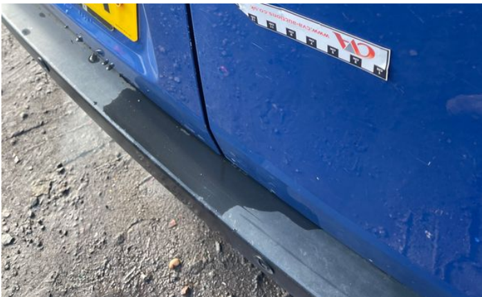
5: Door osf Dented With Paint Damage
