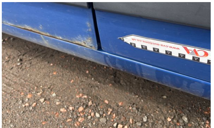
6: Qtr Panel osr Dented Over 30mm
