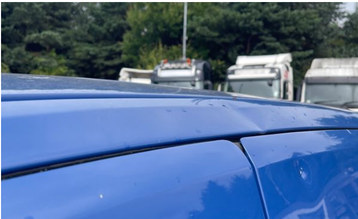
9: Wing nsf Dented With Paint Damage
