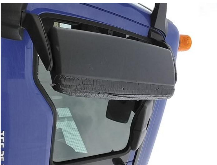
7: Door Mirror Assy nsf Broken Replace
