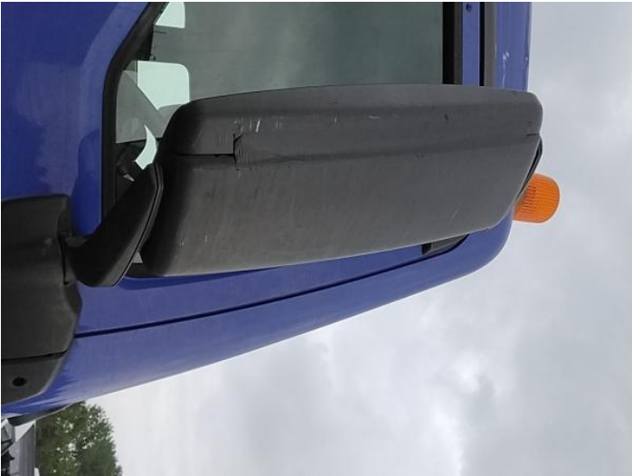
10: Door Mirror Assy osf Broken Replace
