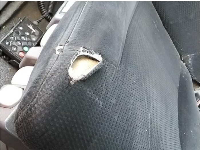
12: Seat Base Cover osf Holed Over 3mm
