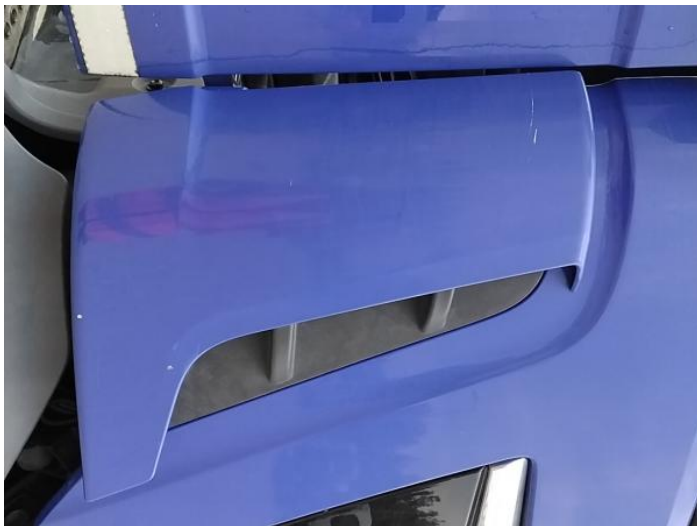
1: Moulding on Wing Scratched (Painted) Over 25mm Thru Paint
