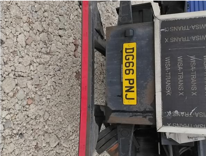
9: Bumper Rear Rusted Over 5mm
