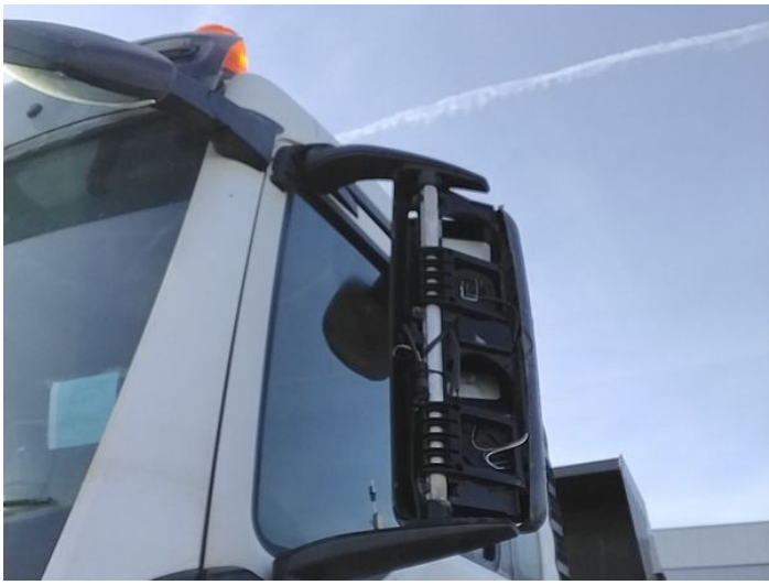
4: Door Mirror Assy nsf Broken Replace
