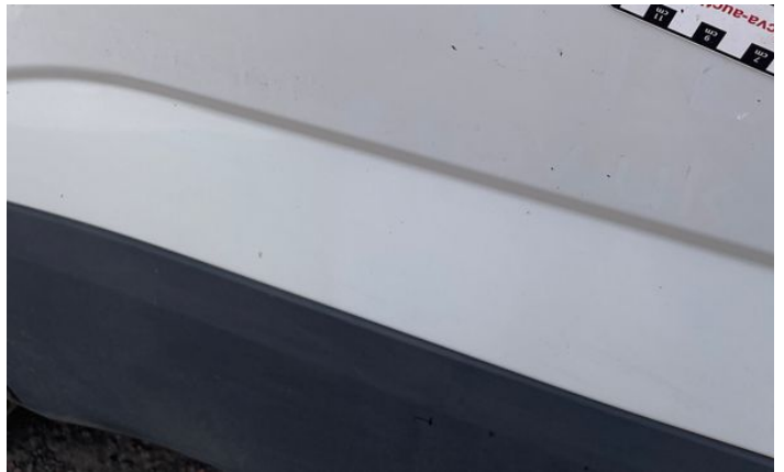
10: Qtr Panel nsr Dented With Paint Damage
