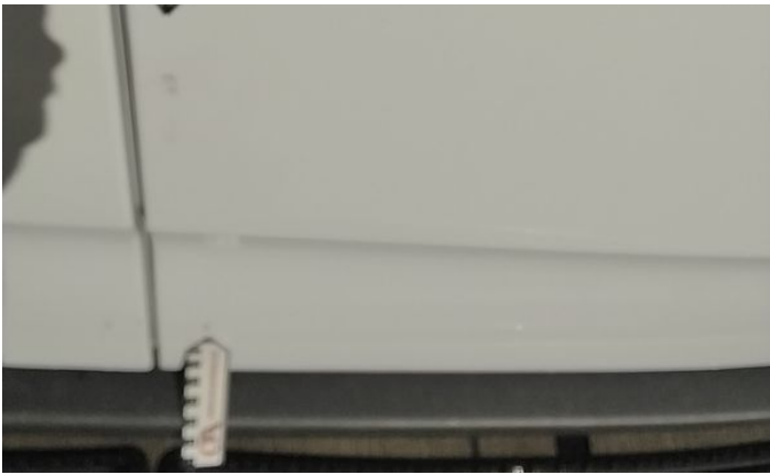
3: Door nsr Scratched Over 25mm Thru Paint
