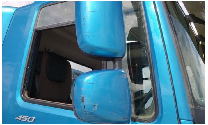
16: Moulding osf Wing Broken Replace
