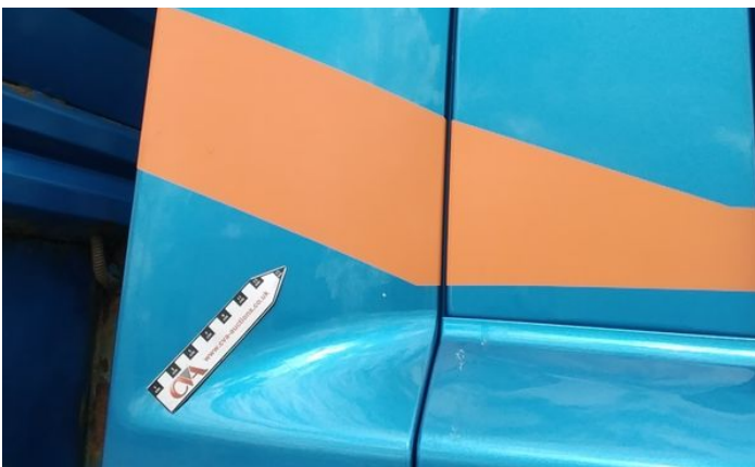
11: Wing Front Arch Extension ns Scratched (Painted) Over 25mm Thru Paint
