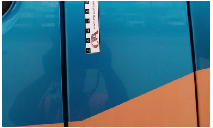
10: Door nsf Scratched Over 25mm Thru Paint
