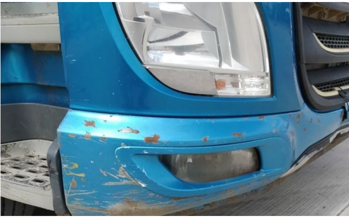
15: Wing Front Arch Extension os Scratched (Painted) Over 25mm Thru Paint
