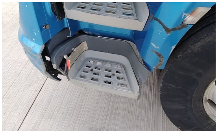
6: Bumper Front Scratched Over 100mm Thru Paint
