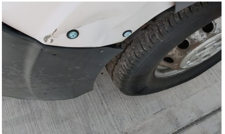
6: Bumper Front Insecure Action Required
