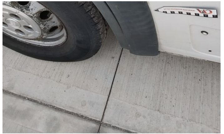
10: Door Moulding nsf Missing Replace
