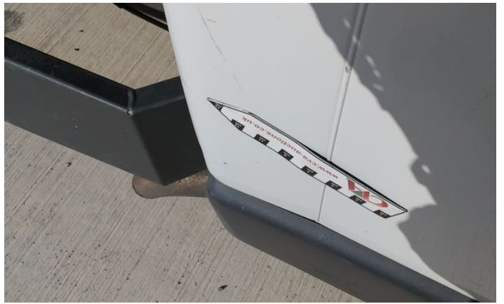
16: Panel Rear Dented With Paint Damage
