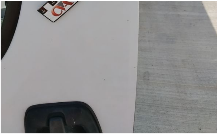
9: Wing nsf Scratched Over 25mm Thru Paint
