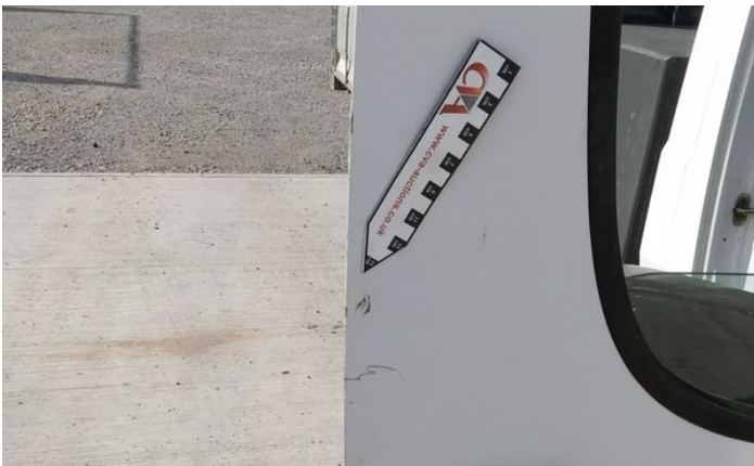
17: B Post os Scratched Over 25mm Thru Paint
