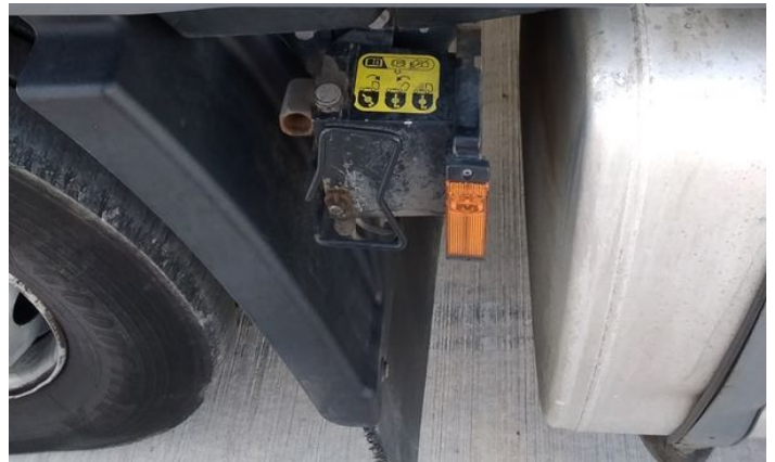
6: Wing Front Arch Extension ns Broken Replace
