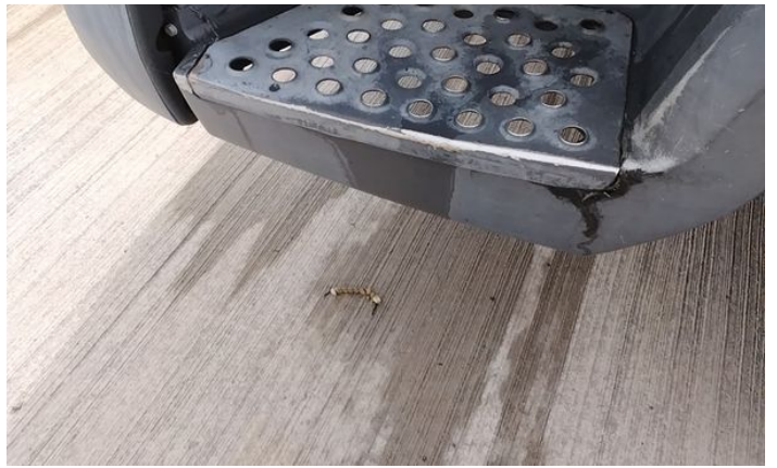
4: Wing nsf Dented With Paint Damage
