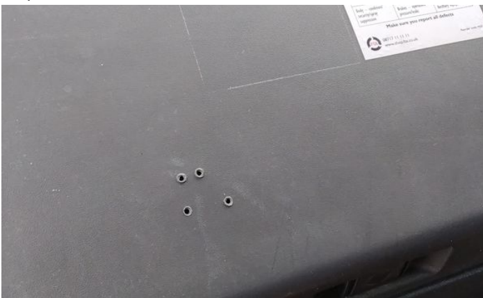
17: Fascia Trim Damaged Replace
