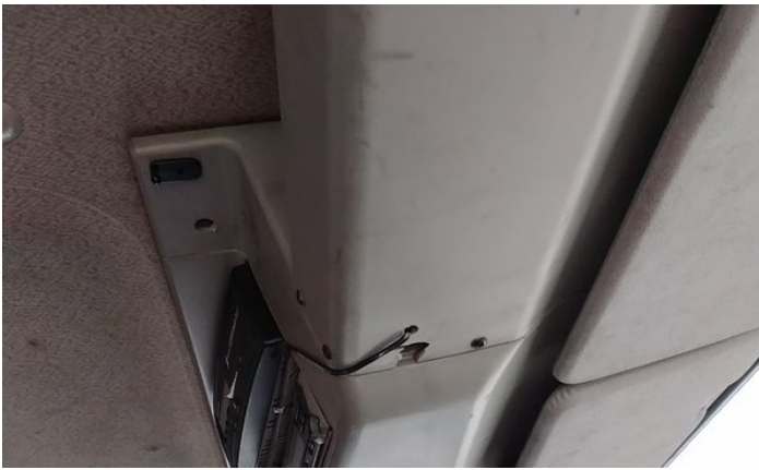
15: Seat Base Cover nsf Holed UpTo 3mm
