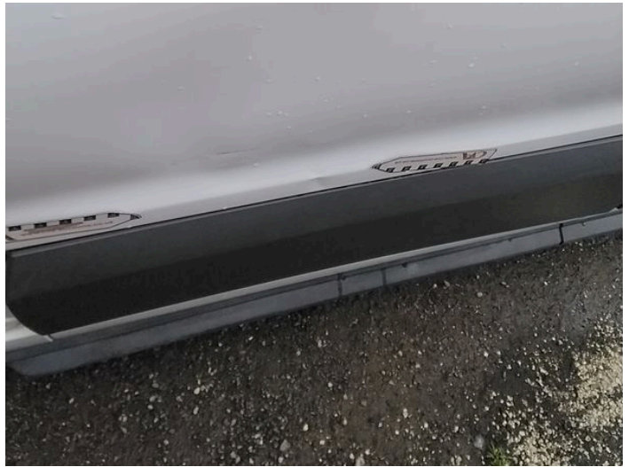
12: Door osr Dented Over 30mm
