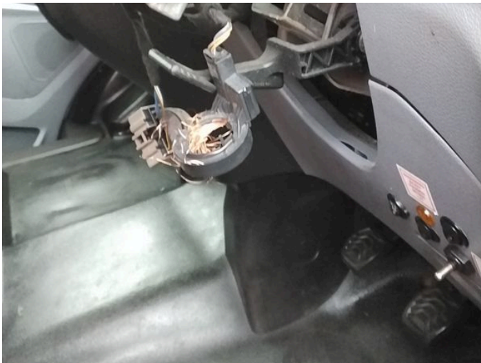
16: Switches And Controls Broken Replace
