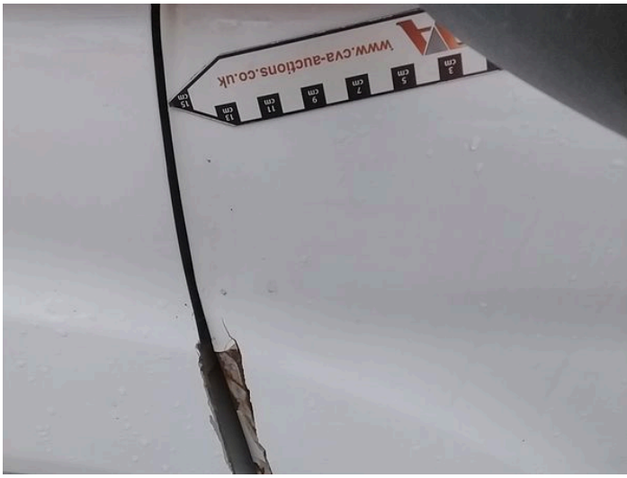
4: Door nsf Dented With Paint Damage
