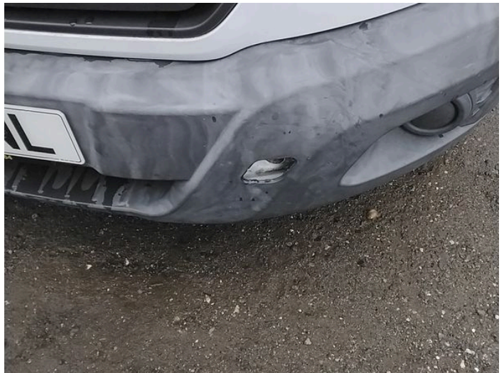
2: Bumper Front Moulding Missing Replace
