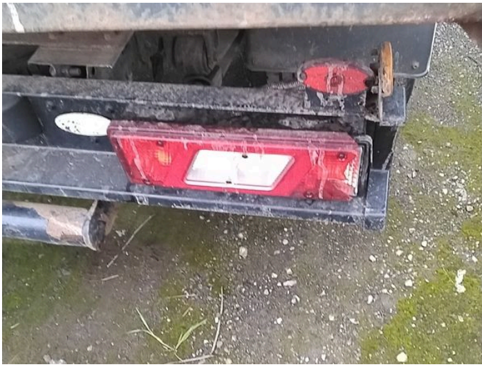
9: Lamp osr Broken Replace
