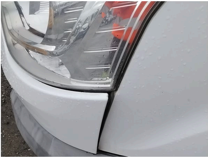
3: Panel Front Cracked Replace
