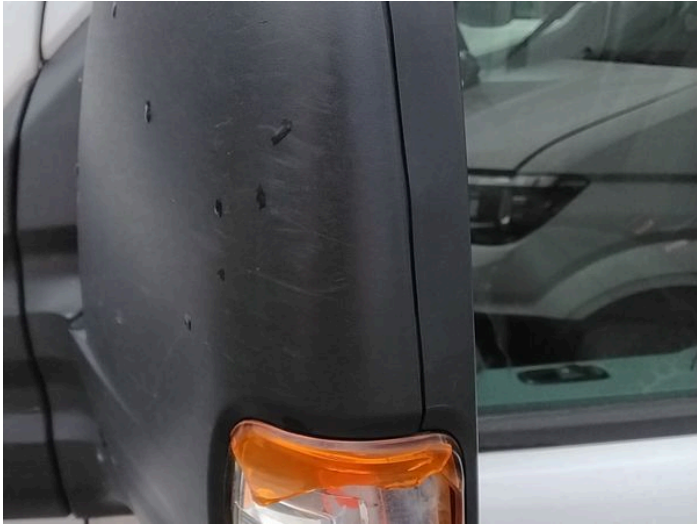
5: Door Mirror Assy nsf Broken Replace
