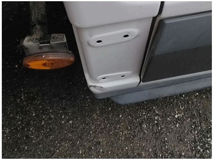
10: Qtr Panel Moulding os Missing Replace
