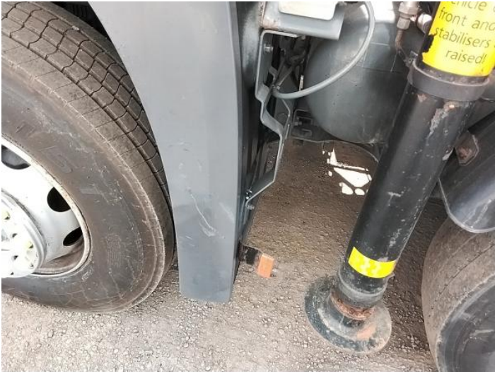
3: Wing Front Arch Extension ns Scuffed (Unpainted) Over 100mm
