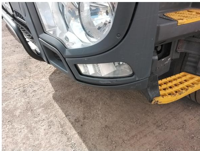
2: Bumper Front Moulding Scuffed (Unpainted) Over 100mm
