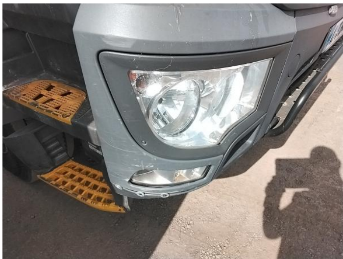
1: Bumper Front Poor Previous Repair Poor Paint
