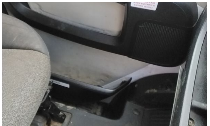
18: Seat Base Cover osf Holed Over 3mm
