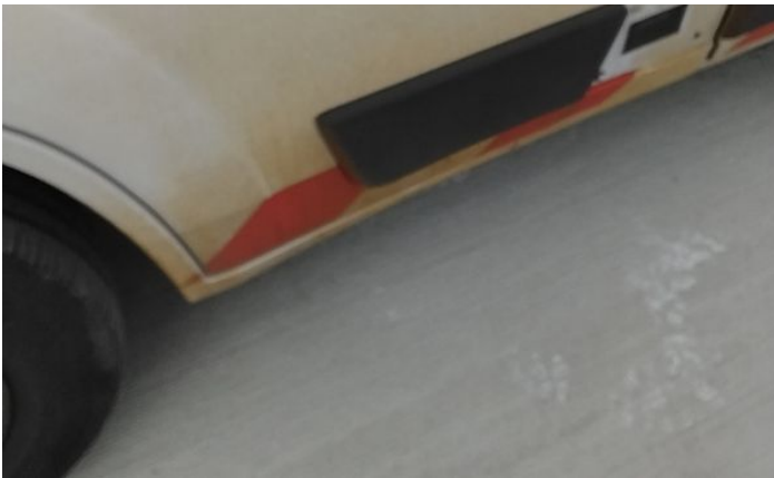
3: Wing nsf Dented With Paint Damage
