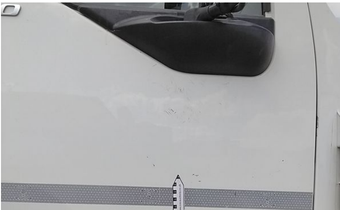
11: Door Mirror Assy osf Scuffed (Unpainted) UpTo 100mm
