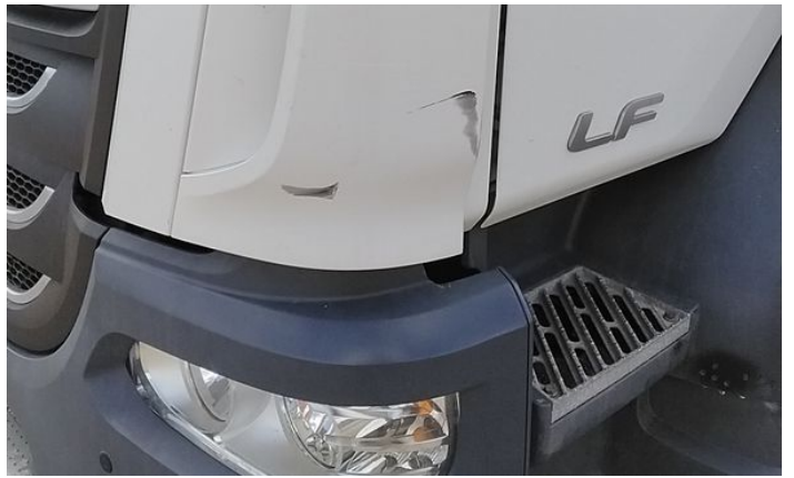
4: Bumper Front Scratched 25 to 100mm Thru Paint
