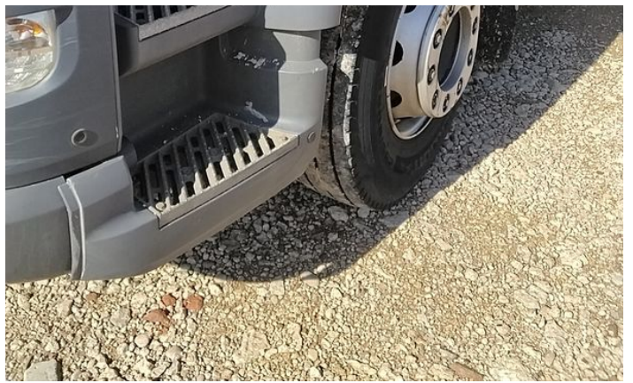
4: Wing nsf Poor Previous Repair Poor Colour
