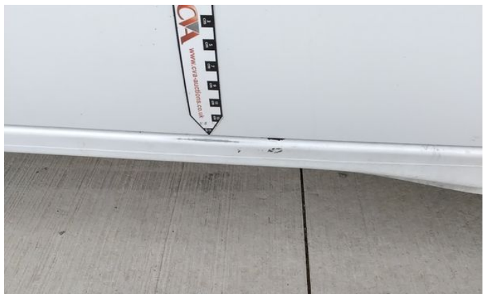
12: Qtr Panel osr Poor Previous Repair Poor Paint
