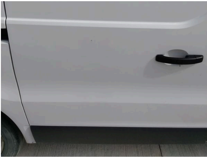
15: Door osr Chipped Over 5mm
