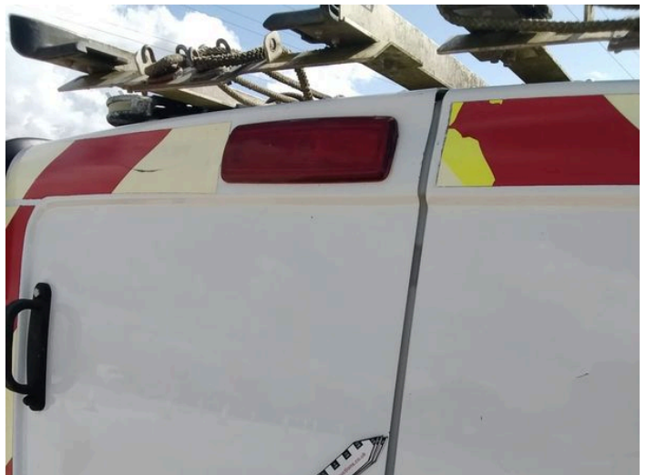
14: Door nsr Chipped Edge Chip
