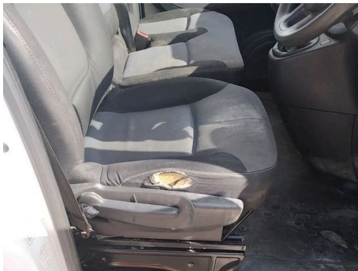
22: Seat Base Cover osf Torn Over 3mm
