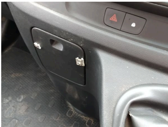
23: Centre Console Front Holed Over 3mm
