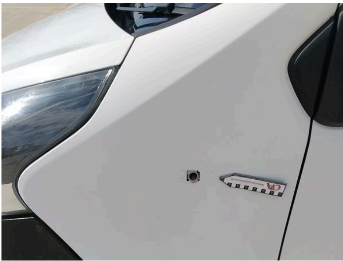
4: Flasher Side Repeater ns Missing Replace
