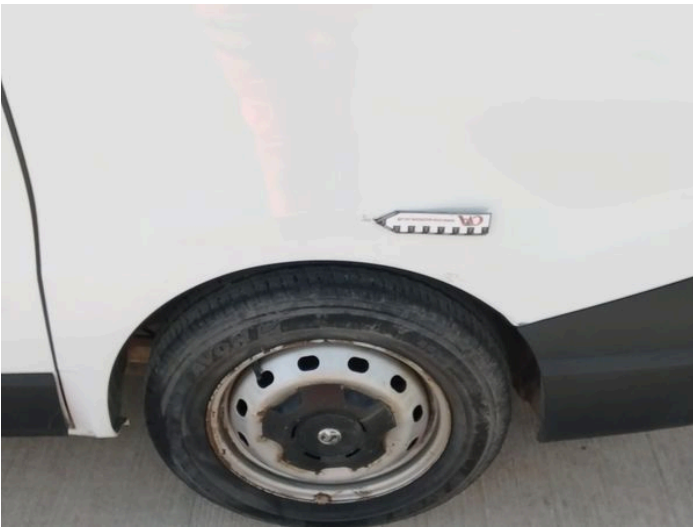
9: Qtr Panel nsr Chipped Over 5mm
