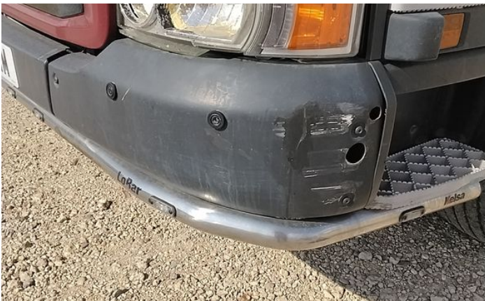
5: Panel Front Cracked Replace
