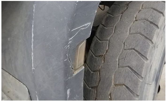
4: Panel Front Scratched Over 25mm Not Thru Paint
