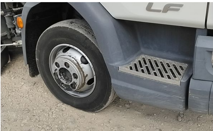
5: Qtr Panel Arch Extension ns Broken Replace
