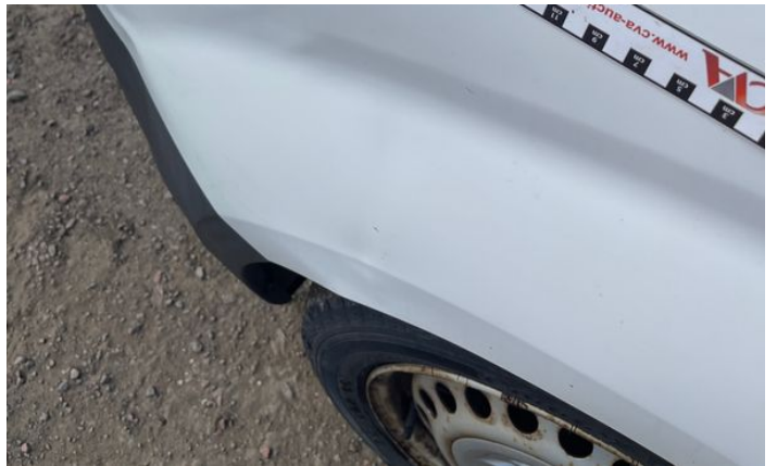
4: Qtr Panel osr Dented With Paint Damage
