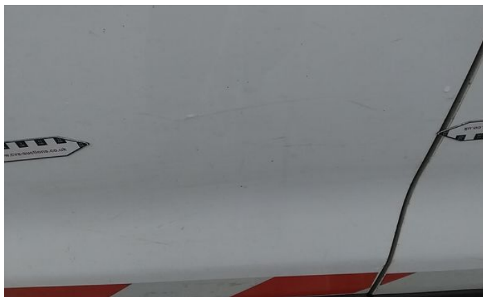
6: Door nsf Scratched Over 25mm Thru Paint
