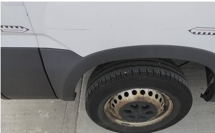
5: Qtr Panel nsr Dented Over 30mm
