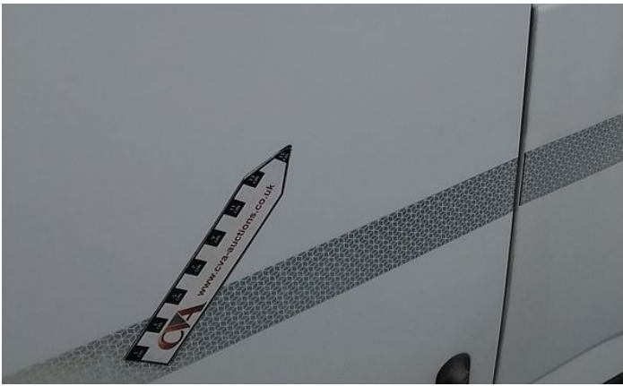
3: Door nsf Scratched Over 25mm Thru Paint
