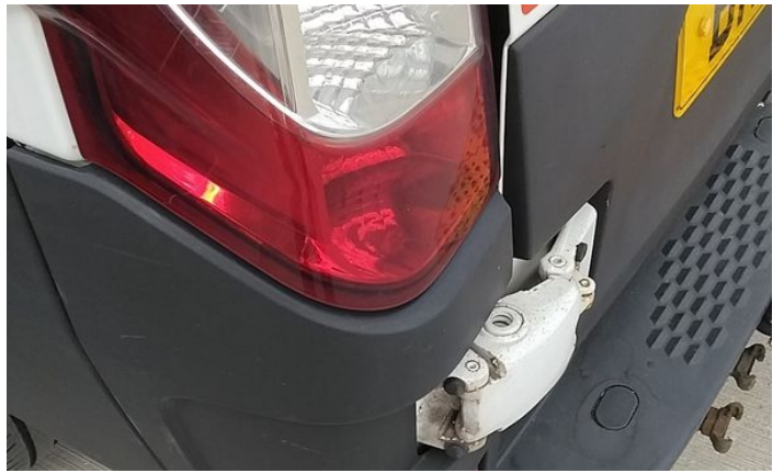
4: Qtr Panel Moulding ns Scuffed (Unpainted) Over 100mm
