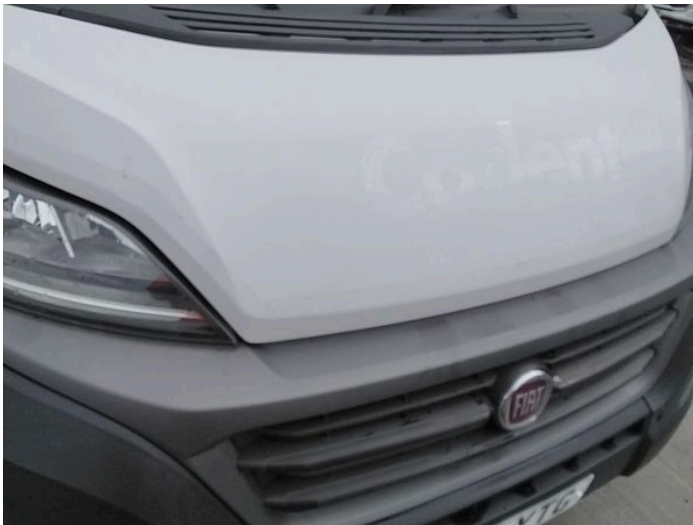
1: Bonnet Chipped Multiple Chips
