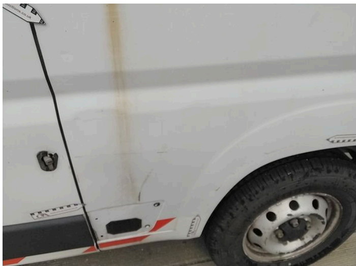
7: Qtr Panel nsr Dented With Paint Damage
