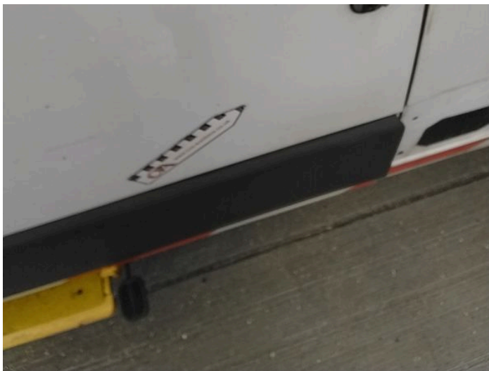
4: Qtr Panel nsr Dented Over 30mm
