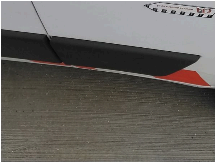
11: Door osf Scratched Over 25mm Thru Paint
