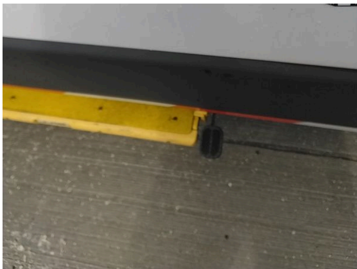
5: Qtr Panel nsr Scratched Over 25mm Thru Paint
