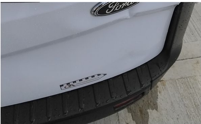
5: Door nsr Dented Over 30mm
