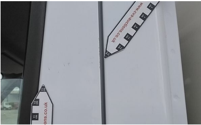
3: Panel Front Scratched Over 25mm Thru Paint
