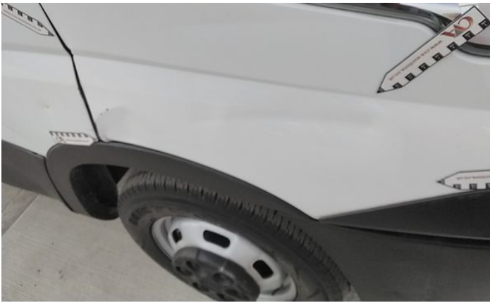
9: Door Moulding osf Scuffed (Unpainted) Over 100mm
