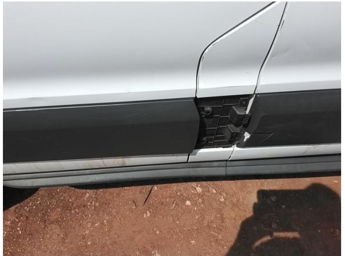
6: Door Moulding nsf Missing Replace
