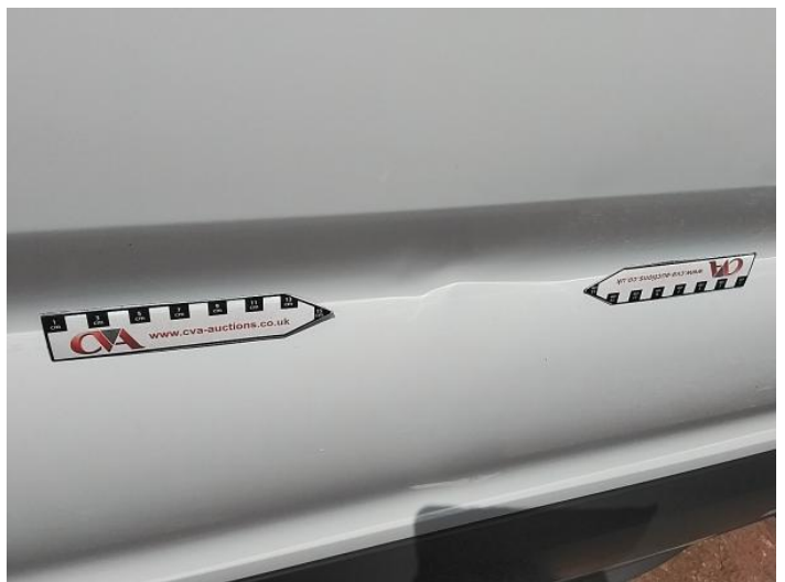
8: Qtr Panel nsr Dented Over 30mm
