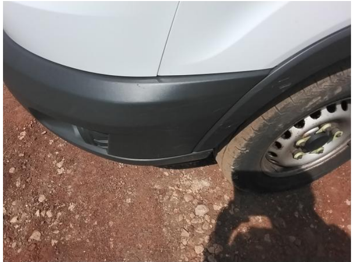
4: Bumper Front Scratched Over 100mm Thru Paint
