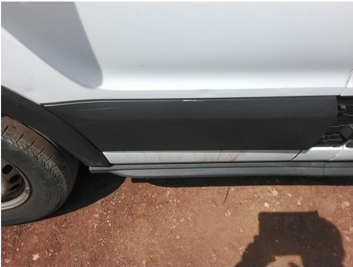
5: Door Moulding nsf Scuffed (Unpainted) Over 100mm
