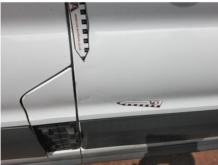
7: Qtr Panel nsr Dented With Paint Damage
