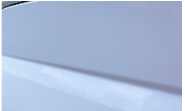
10: Door nsr Dented With Paint Damage
