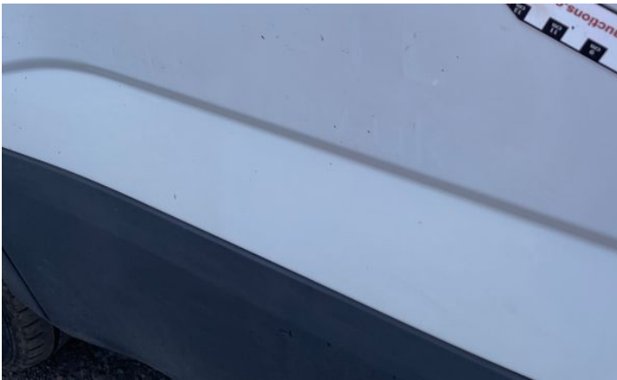
9: Qtr Panel nsr Dented With Paint Damage
