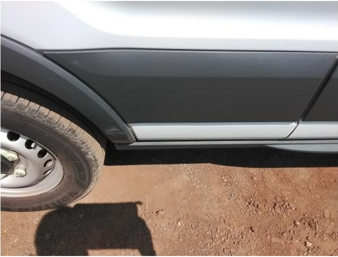
9: Qtr Panel Moulding os Scuffed (Unpainted) Over 100mm
