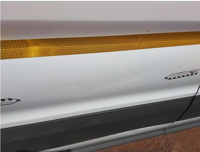
11: Qtr Panel osr Dented With Paint Damage
