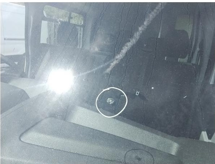
13: Screen Front Chipped Over 10mm
