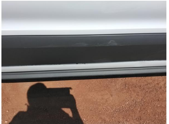
12: Qtr Panel Moulding os Scuffed (Unpainted) Over 100mm
