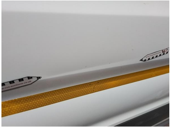
10: Qtr Panel osr Dented Over 30mm
