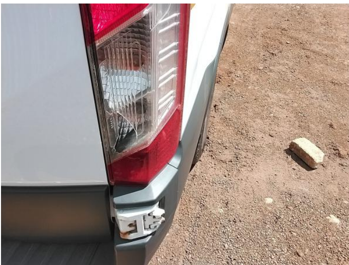
7: Lamp osr Broken Replace
