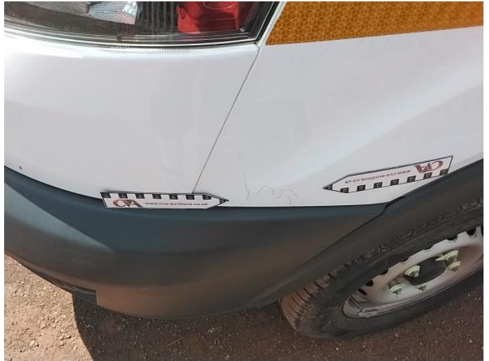
4: Wing nsf Scratched Over 25mm Thru Paint
