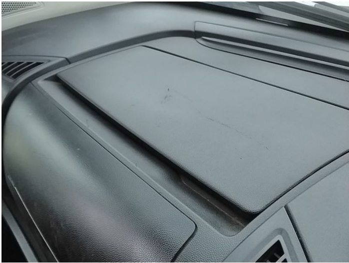
11: Fascia Panel Scuffed Over 25mm
