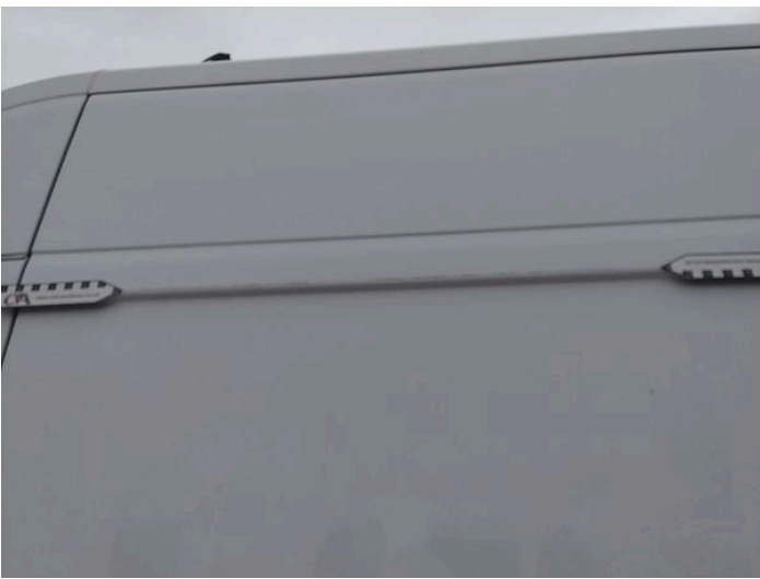
4: Qtr Panel nsr Scratched Over 25mm Thru Paint
