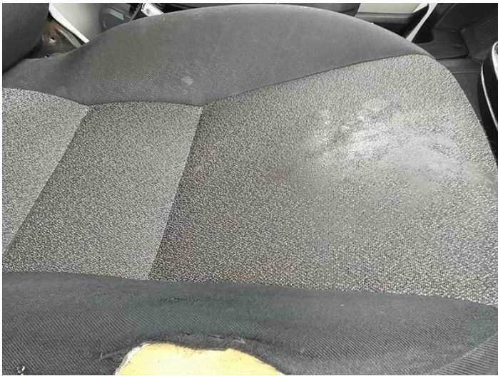
9: Seat Base Cover osf Holed Over 3mm
