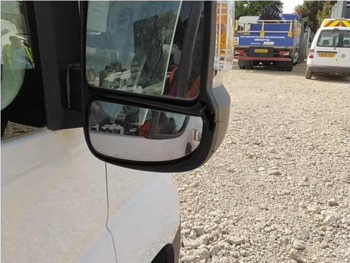
18: Door Mirror Assy osf Broken Replace
