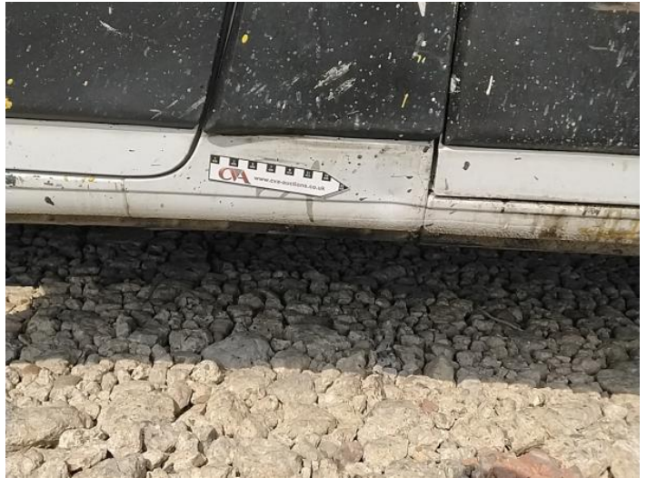
10: B Posts Dented Between 10mm + 30mm
