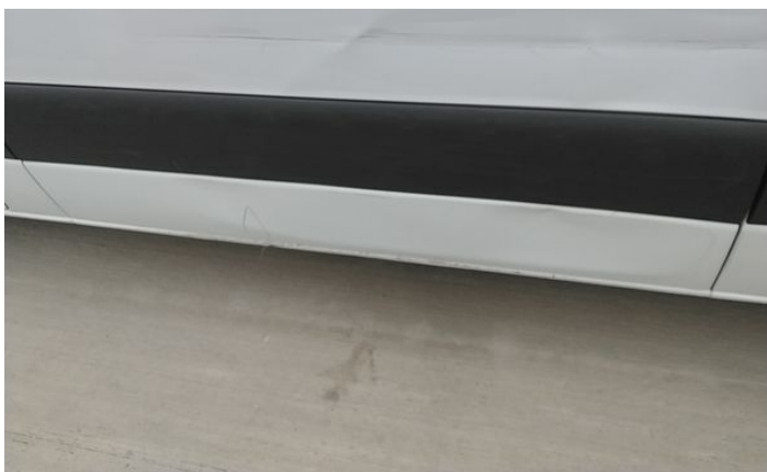
3: Qtr Panel nsr Dented Over 30% Of Panel
