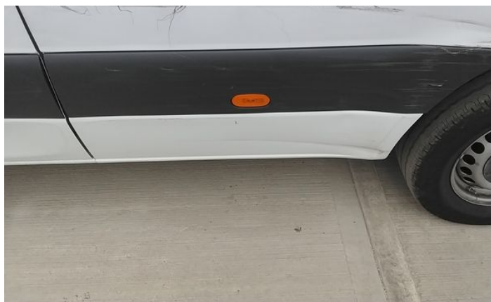
4: Qtr Panel nsr Dented Over 30% Of Panel
