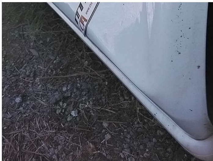
6: Panel Rear Dented Over 30mm
