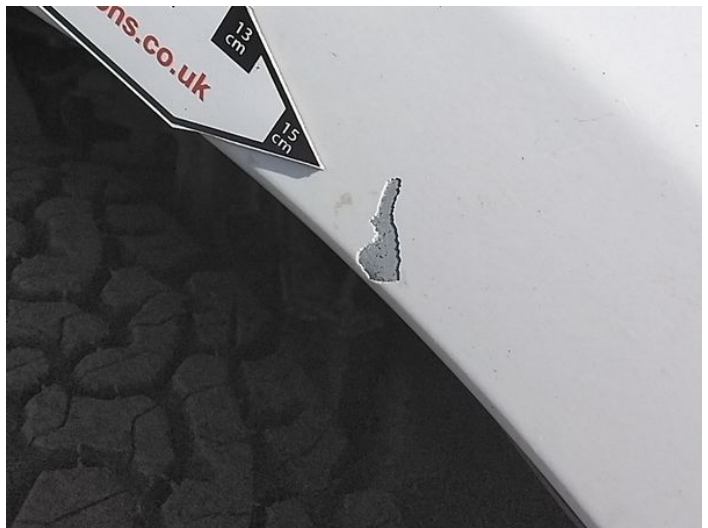
10: Wing nsf Chipped Over 5mm
