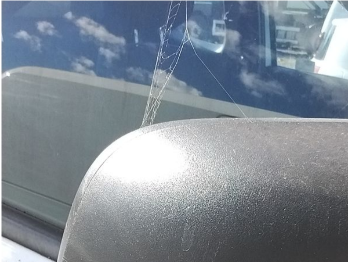
1: Door Mirror Assy osf Scuffed (Unpainted) Over 100mm
