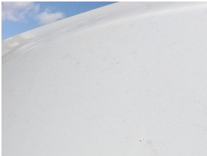
11: Wing nsf Chipped Over 5mm
