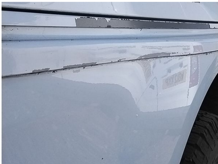
3: Panel Rear Chipped Multiple Chips
