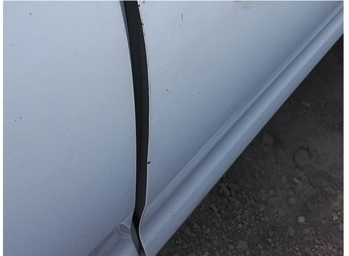
2: Door osf Chipped Edge Chip
