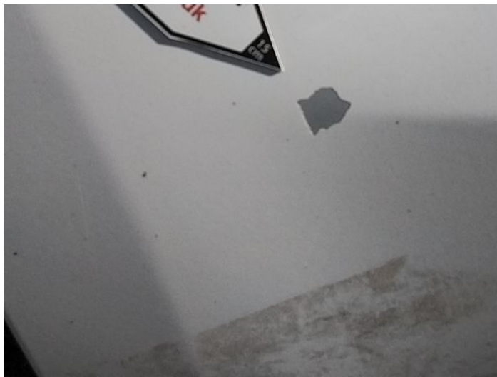
9: Wing nsf Chipped Over 5mm
