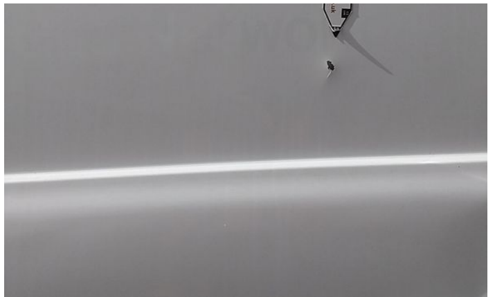
6: Door nsf Dented Between 10mm + 30mm
