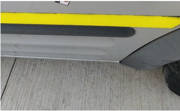
9: Door nsf Scratched Over 25mm Thru Paint
