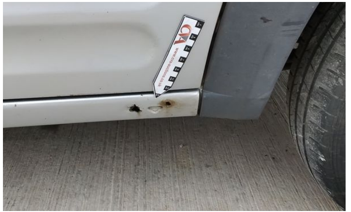
10: Door nsf Dented Over 30mm
