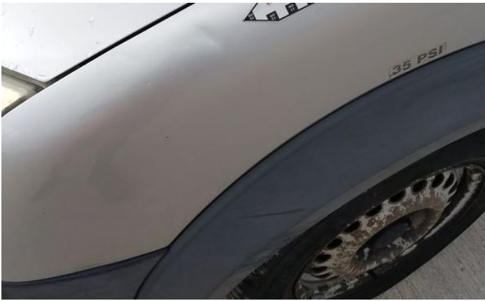
3: Bumper Front Scratched Over 100mm Thru Paint
