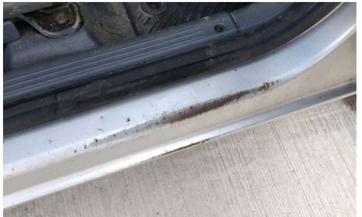
22: Fascia Trim Damaged Replace
