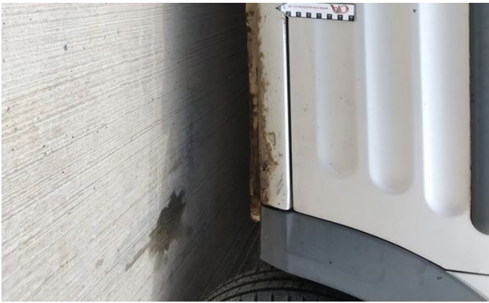
15: Qtr Panel osr Scratched Over 25mm Thru Paint
