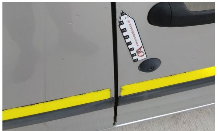
16: Qtr Panel osr Scratched Rusted
