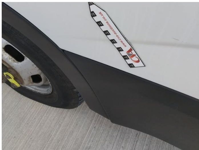
6: Door nsf Dented Over 2 UpTo 10mm
