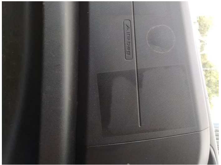
22: Centre Console Front Holed Over 3mm
