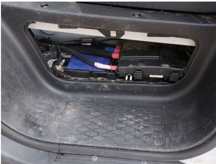
25: Fascia Panel Missing Replace
