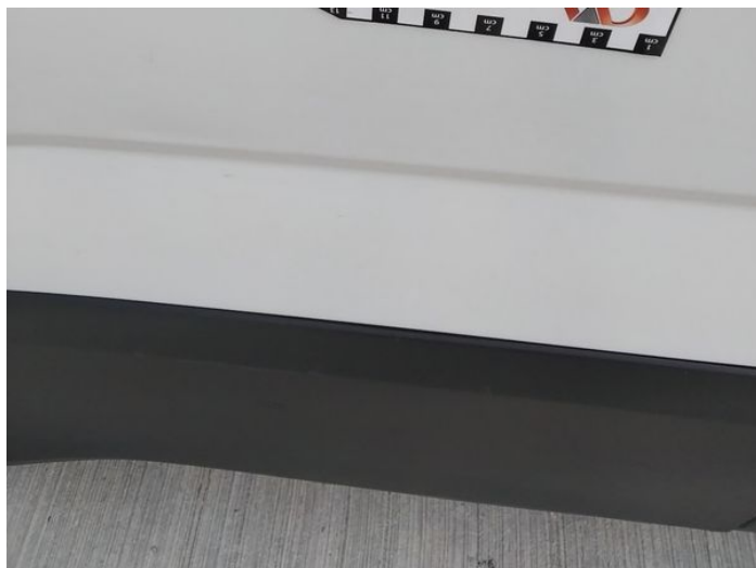
8: Door nsf Scratched Over 25mm Thru Paint
