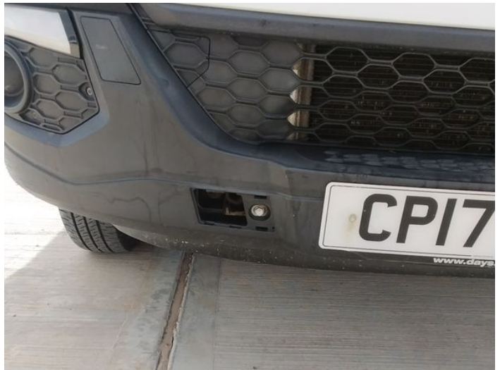
2: Front TowEye Cvr Missing Replace
