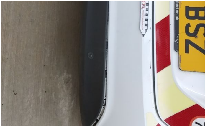
9: Qtr Panel nsr Chipped Multiple Chips
