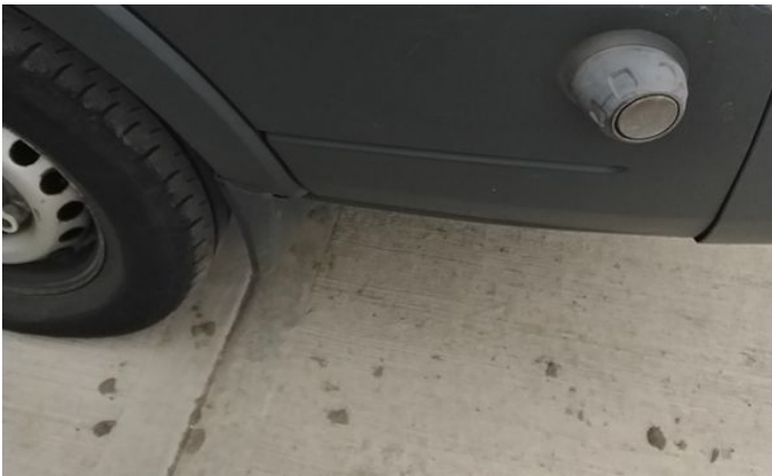
9: Qtr Panel nsr Chipped Multiple Chips
