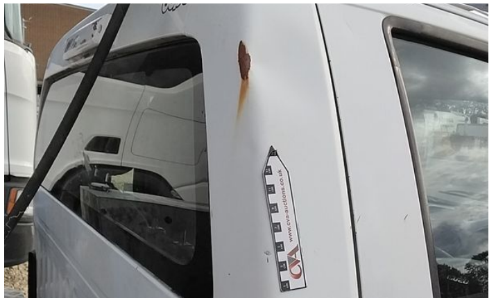
6: Door nsf Dented With Paint Damage
