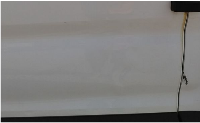
3: Panel Front Scratched UpTo 25mm Thru Paint
