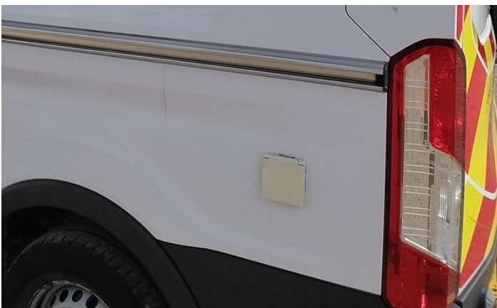
5: Door nsr Dented Over 30mm
