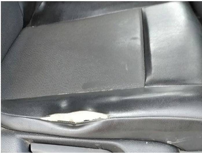
9: Seat Base Cover osf Torn Over 3mm
