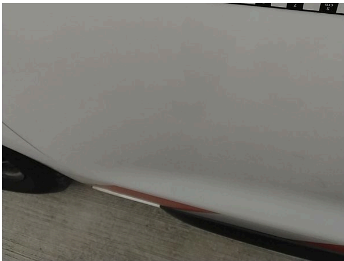
4: Door nsf Dented With Paint Damage
