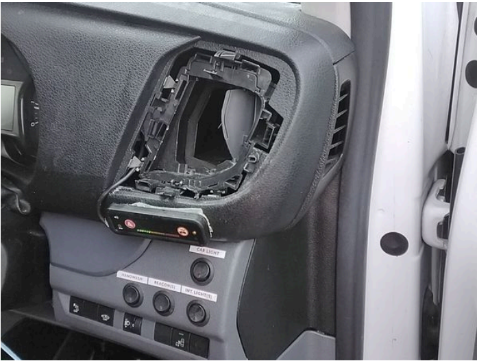
12: Air Vents osf Missing Replace
