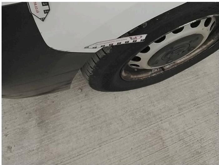
3: Wing nsf Scratched Over 25mm Thru Paint
