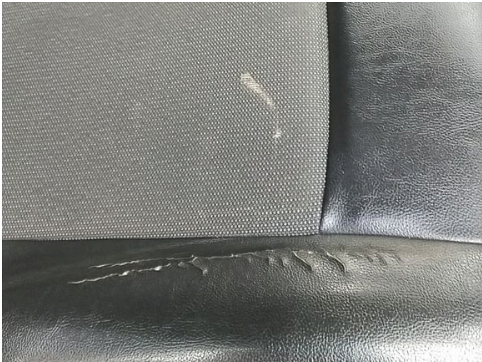
13: Seat Base Cover osf Torn Over 3mm
