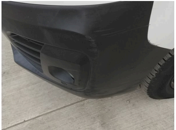
2: Bumper Front Scratched Over 100mm Thru Paint
