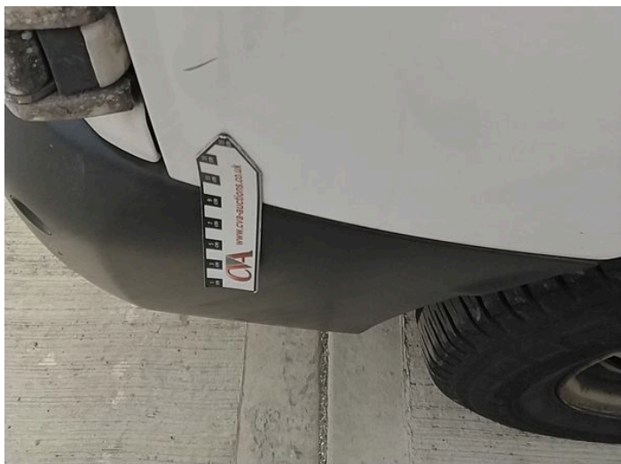
7: Qtr Panel osr Dented With Paint Damage
